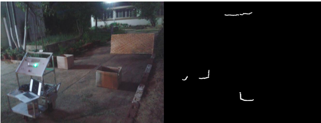
Figure 11: Obstacle Detection using 2D Lidar
